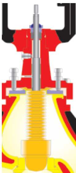
Fig. 1 - lined globe valve Primary stem sealing by PTFE-bellow. Secondary seal by additional safety PTFE-Graphite packing
