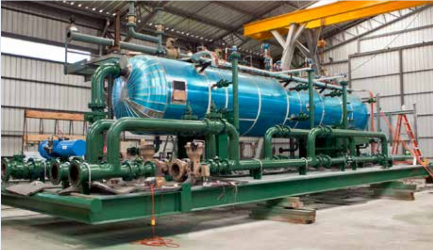
Typical three-phase oil separator fitted with SAMSON valves
