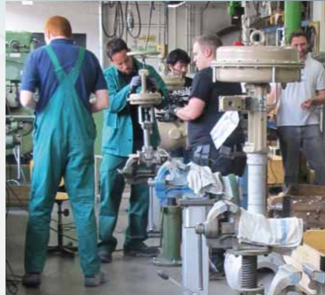
The committed team of service technicians work together to overhaul valves at a steam cracking plant.
