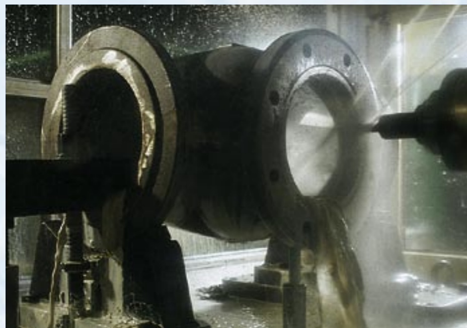
CNC machining center with high positioning precision and cutting capacity is able to handle the complete machining process required to produce valve bodies.
