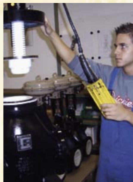
A valve bonnet, with PTFE plug and bellows seal attached, is assembled at Pfeiffer.
