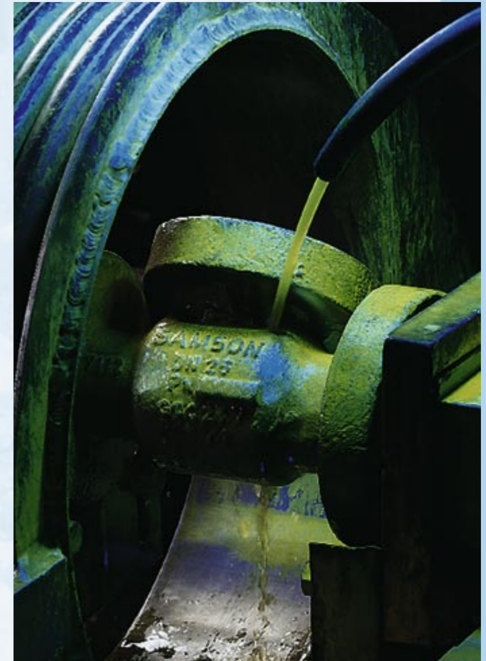
The fluorescent iron particles settle in any cracks of the workpiece in the magnetic particle test and are made visible in ultraviolet light.
