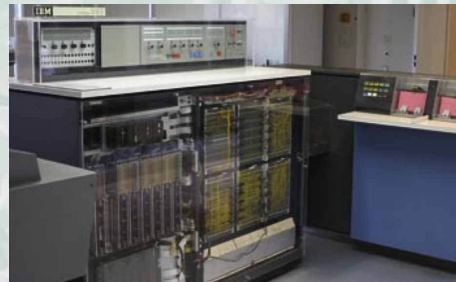
The 16 KB memory of the first mainframe computer at SAMSON, an IBM S/360-20 computer, was sufficient to cope with the entire accounting transactions by feeding punch cards into the computer.
