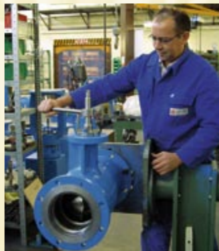
The precise machining of all valve parts plays a key role in the production of rotary plug valves at VETEC to ensure reliable functioning and a long service life.
