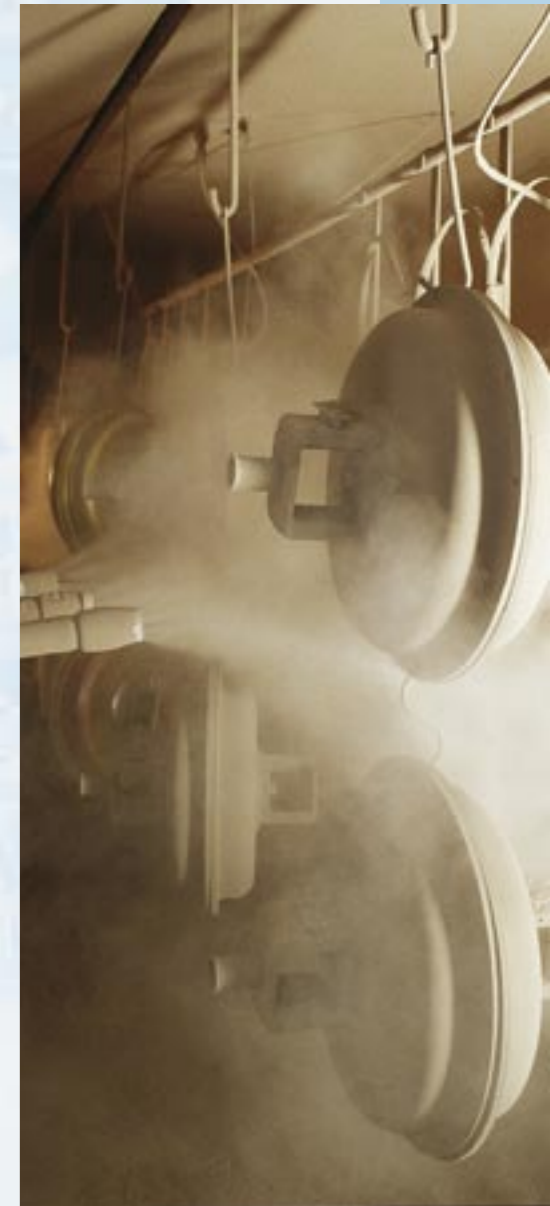
The standard paint coating is applied by electrostatic spray procedure. Coats to meet special customer specifications and repairs are done by hand.
