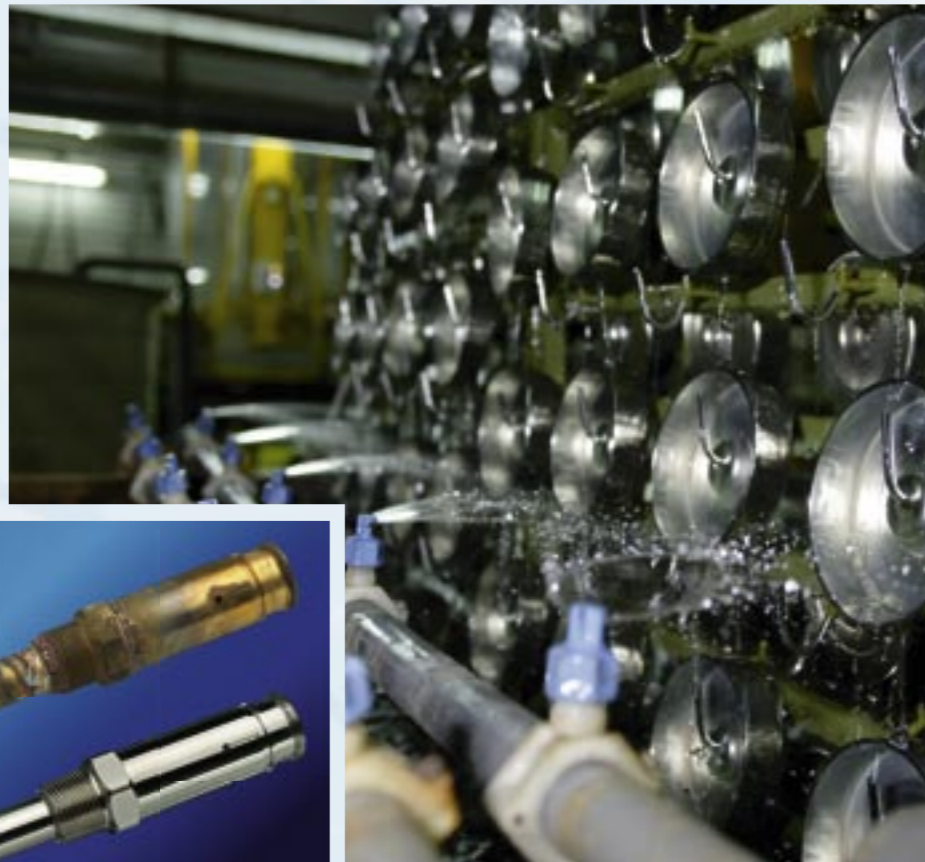
Corrosion protection is a priority at SAMSON. The surface of parts is given the best finish with the appropriate technique in the automated electroplating plant.
