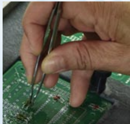
Not all components can be automatically fitted onto printed circuit boards. The components are soldered on to the bottom of the board in a wave bath.
