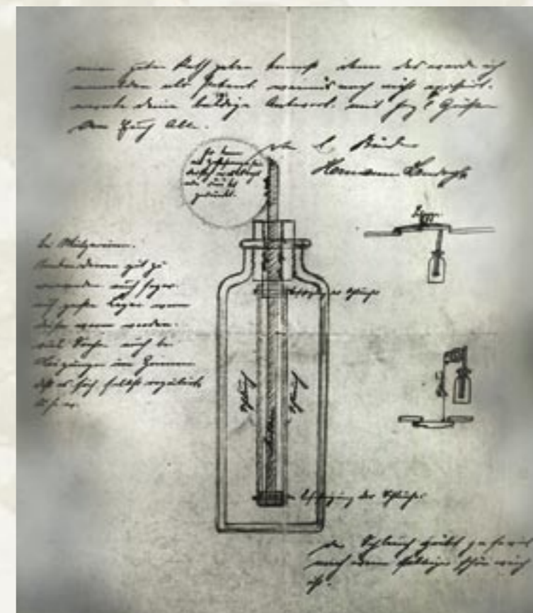
Hermann Sandvoss put the principle of liquid expansion to use in combination with a reliable metal bellows to regulate the temperature.
