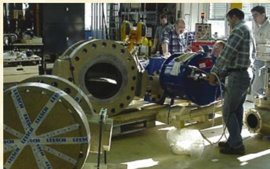
Triple offset butterfly valves from LEUSCH intended for a SAMSON project are extensively tested before their dispatch.
