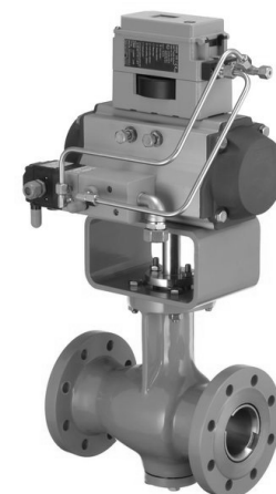
Type 82.7 Rotary Plug Valve with Type AT Rotary Actuator and Type 3730 Positioner
