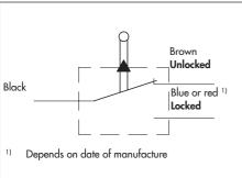
Fig. 4: Circuit diagram for signal transmitter
