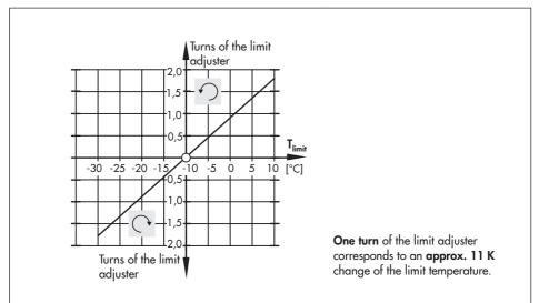
Fig. 7-1: Adjustment diagrams of Type 2040, with temperature limit T<sub>limit</sub> = −10 °C (point at which the regulator is fully closed)
