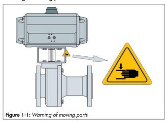
There is a danger of crushing due to the rotary movements of the actuator- and control shaft when reaching into the yoke as long as the pneumatic power is connected to the actuator. At the operator's request, a warning note can be attached to the valve.
