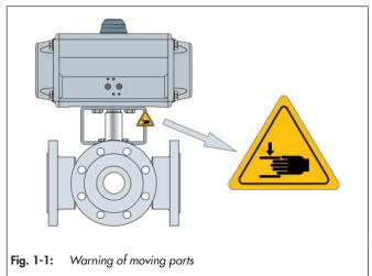
There is a danger of crushing due to the rotary movements of the actuator- and switching shaft when reaching into the yoke as long as the pneumatic power is connected to the actuator. At the operator's request, a warning note can be attached to the valve.
